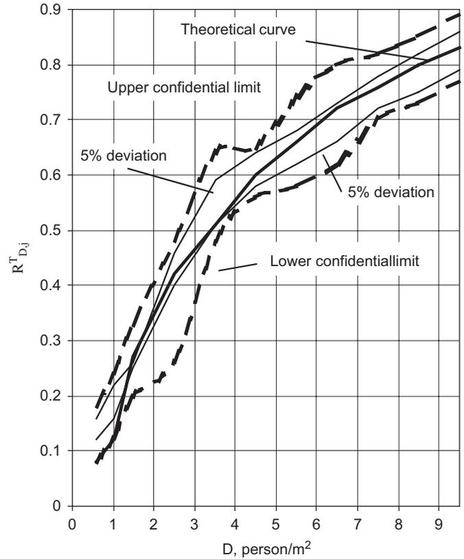
Fig. 5. An example of relation  $R_T = f(D)$  approximation: horizontal path in buildings.
